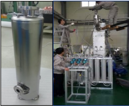
QWR SC Cavity & its Cryomodule
